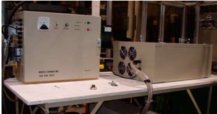
2 Cartridge Annealing Systems of 30-50 kW - 20 kHz each
