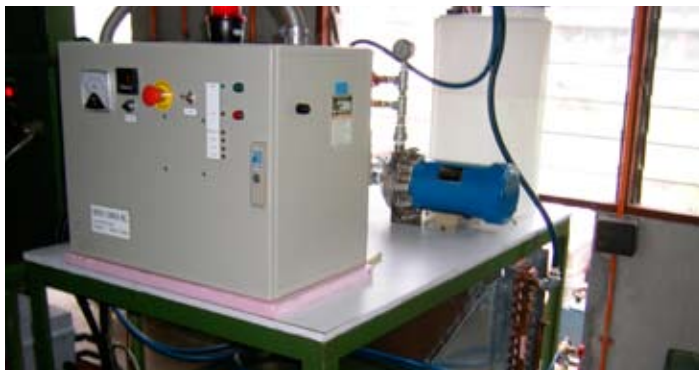
Cartridge Annealing with a 50 kW – 20 kHz Induction System
