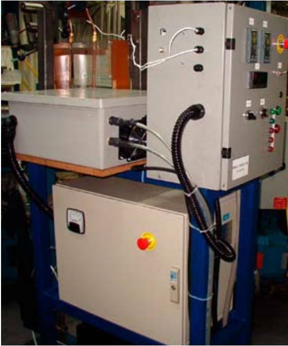
MP Series, 40 kW - 20 kHz for preheating cable
