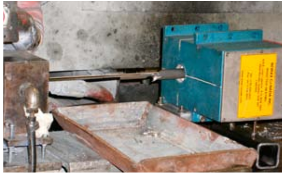
Magnetic Zinc Wiping Systems for galvanized wires and tubes
